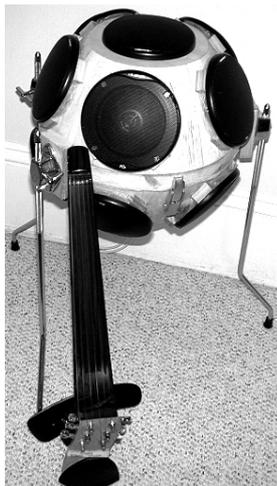
Figure 1: an early spherical speaker with electric violin
